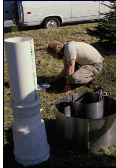
Double-Ring Infiltration Tests
